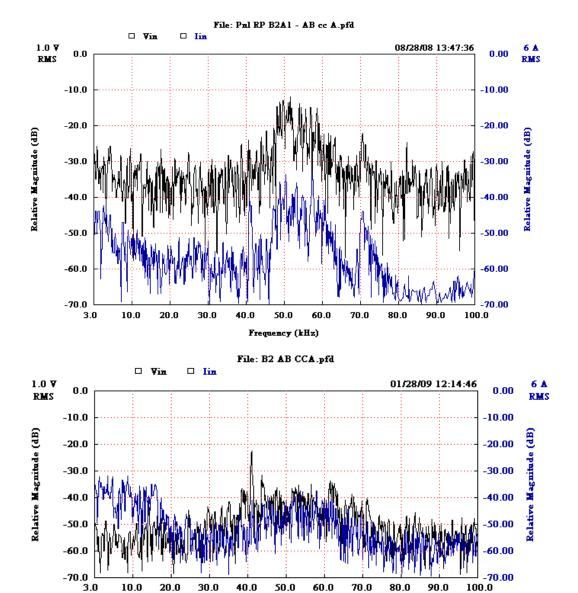
RP B2 Phase A to Phase B was extremely noisy with peaks of the base line as high as -12 dB. After EP Filter Protector was installed the baseline clearly flattened out with the base line of the voltage (black in color) now at -35 dB. This is a reduction of -23 dB or a noise power factor reduction of 20.5.
