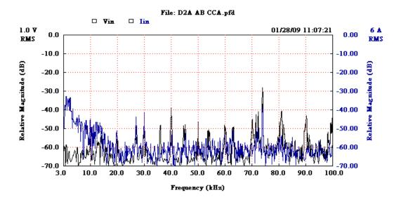
Panel D2A Phase A to B before filters showed noise levels on voltage line basically around the -35 dB marker. After filter was installed, this base line dropped down to earth noise level between - 65 and -70 dB. Basically a reduction of the power of the noise by a factor of 35.
