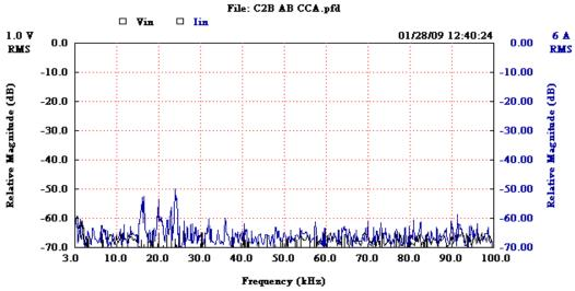
DP C2B Phase AB before filters showed a very strong high frequency noise presence on the power distribution lines as high as -28 db. After the filters were installed, the voltage dropped down to a -68 db baseline, which is basically earth noise. This filter reduction was a drop in the noise by a power factor of 40.
