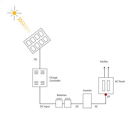
Figure 3: Solar Generation Facility
