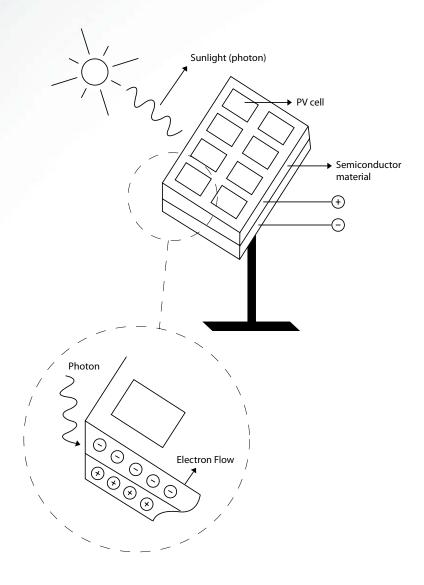
The current generated by this process is DC. The voltage of the solar power is small in magnitude, approximately 48VDC. However, the distribution system is designed for AC. Industrial and commercial loads require AC in order to function. This means the power generated by the solar cells is not useful for industrial applications.
