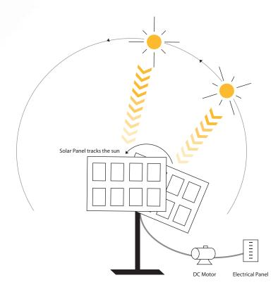
Figure 2: Active solar tracking system.
