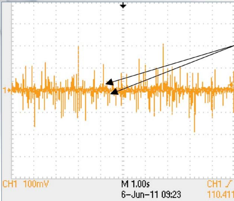
*The thickness of the hash was significantly reduced after installing EP's waveform correctors. This shows that installing EP units decreases the shaft voltage amplitude.*
