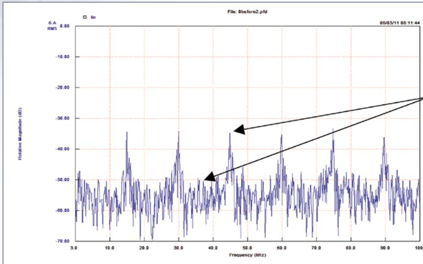
*The bearing current peaks reach approximately -35dB while the noise is approximately -50dB.*
