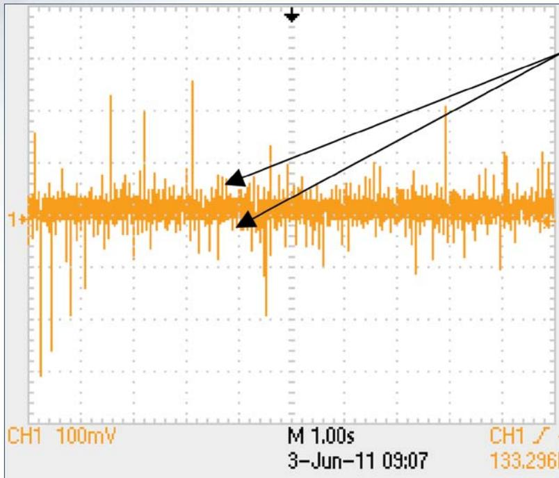
*Figure 7 shows significant levels of voltage noise. There are regular peaks and significant hash. The thickness of the hash shown with the arrows is significant enough to cause bearing currents in the motor.*
