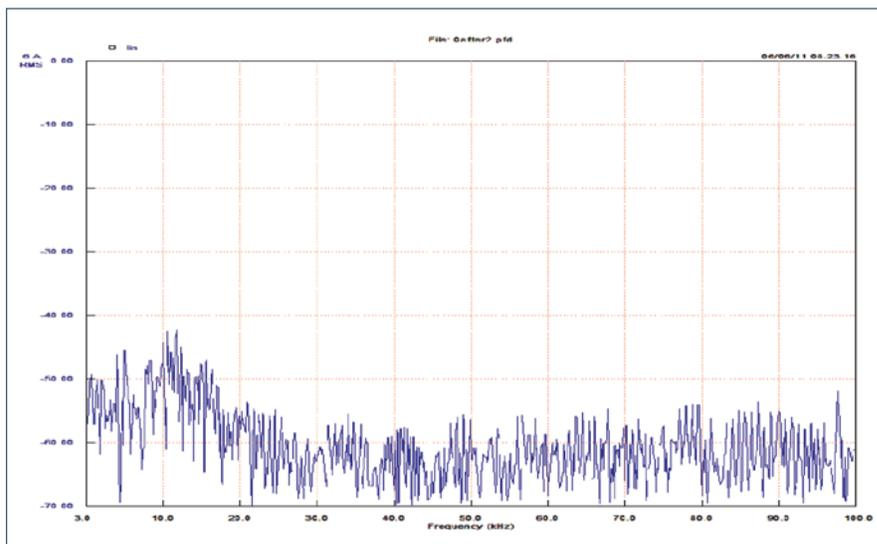
After installing EP's waveform correctors, all of the bearing current peaks were removed. The noise was also reduced to less than -55dB.
