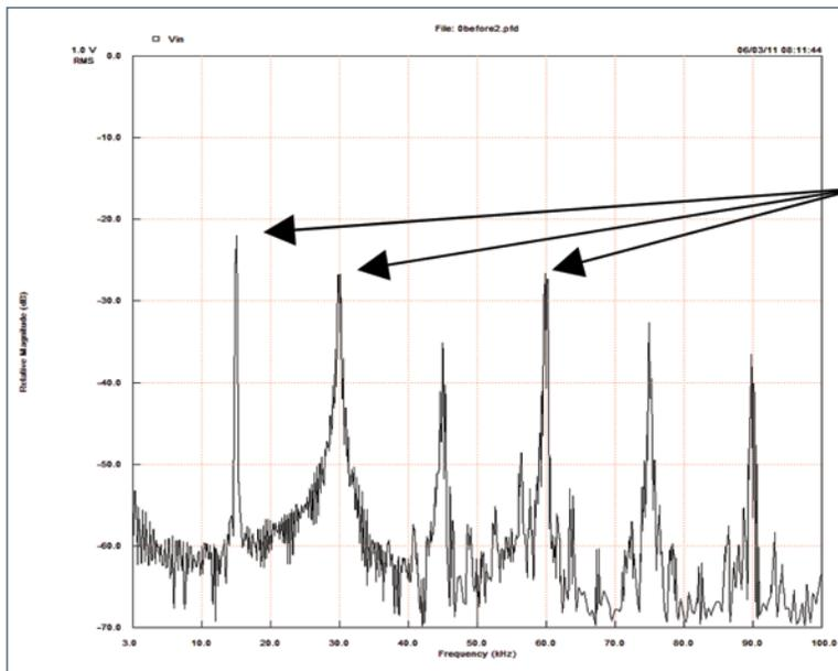
*The bearing voltage high frequency noise reaches approximately -22dB at 15kHz and approximately -27dB at 30kHz and 60kHz.*
