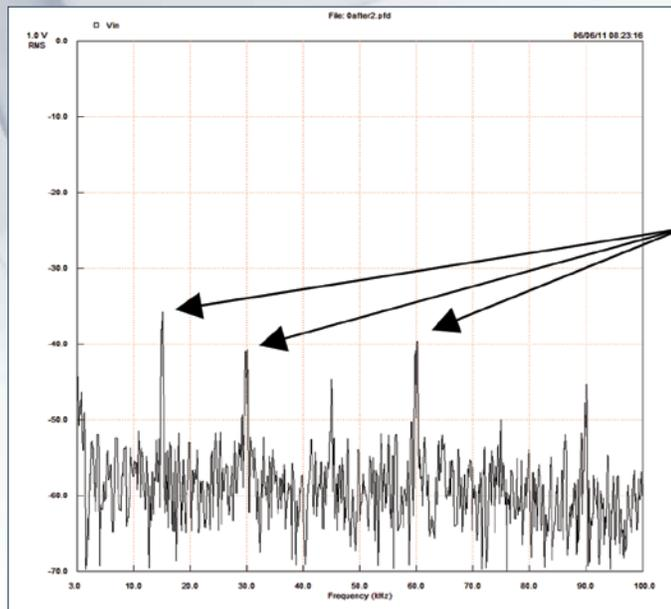
After installing EP the common mode voltage is significantly reduced. The peaks were reduced by approximately -14dB when compared to the readings in figure 3.
