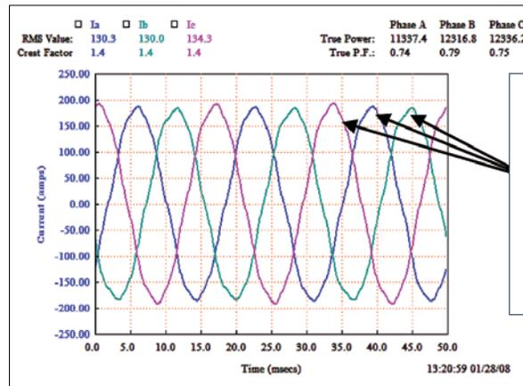
**Figure 4:** After installing EP, skin effect and proximity effect are removed. Balancing the current levels for phases a, b & c.
