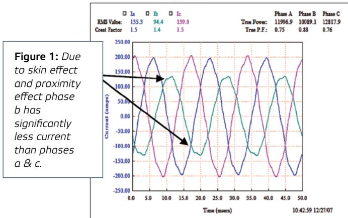
**Figure 1:** Due to skin effect and proximity effect phase b has significantly less current than phases a & c.
